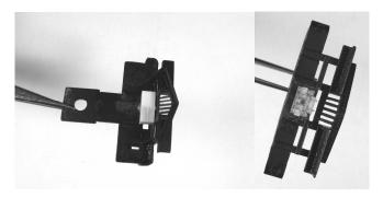
Now all that is left to do is apply a little paint and put it all back together. Clip the mounting pin off below the pocket and flatten it to prevent it from inadvertently coming out.
