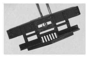
The photos below show the pocket as mounted in the modified locomotive pilot. Note that the 0-80 mounting screw is not really required, but installed just to be "proper".
