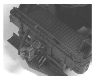
The Sergent Engineering Model ES1P87 finally allows the modeler quit compromising! This kit contains an operational scale size coupler and a highly detailed insulating coupler pocket. These
